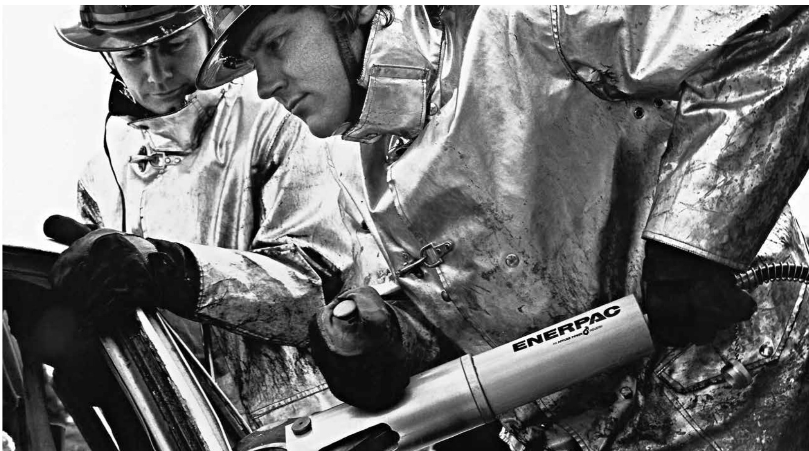
Grant (right) and colleague, operating the Jaws of Life, used to pry apart wreckage of crashed vehicles in order to free trapped people, 1978
